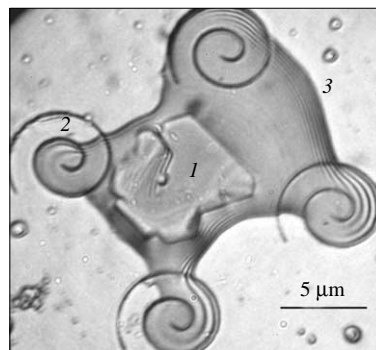
Figure 4 Formation of anisotropic droplets of an aqueous solution with crystallising L-valine (1) on chiral periodic elements of a superficial relief (2). Lines (3) are observed due to light interference in the liquid film (edge of the droplet) of different thickness.
